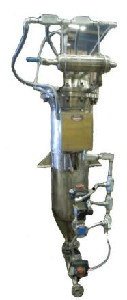
Additionally an 8" dia x 33.31" OAL Hastelloy C276 Filter Housing was also supplied.
