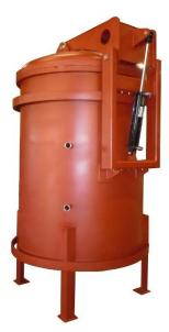
The vessel required a 5 torr or better leak rate. The test procedure isolated the vessel from the vacuum pump with a ball valve with the pump turned off. A gauge was monitored and recorded vacuum for ten minutes. The vacuum loss, based on the vessel size and empty state, after ten minutes was fewer than 2.5%.
