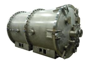
The vessel required a calibrated leak rate of 1.4 x 10-7 scc/He/sec. The test procedure isolated the vessel from the vacuum pump with a ball valve with the pump turned off. A gauge was monitored and vacuum readings were recorded.
